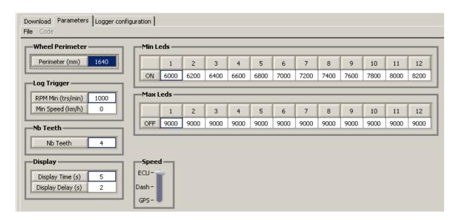
This tab sets all parameters available in the logger, including the display (for dashes).
