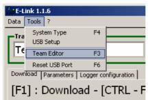
Every device is identified by its own serial number, and the download is enabled by entering a pincode associated to it. The team editor allows to associate a serial number to a driver name and a pincode.
