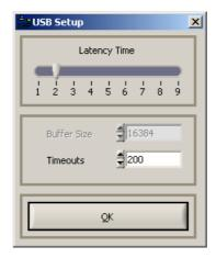
The default values should work correctly, but it could be necessary to raise the latency (to 3 or 4) and the timeouts (to 250-300ms) on some computer. This will affect the download speed.
