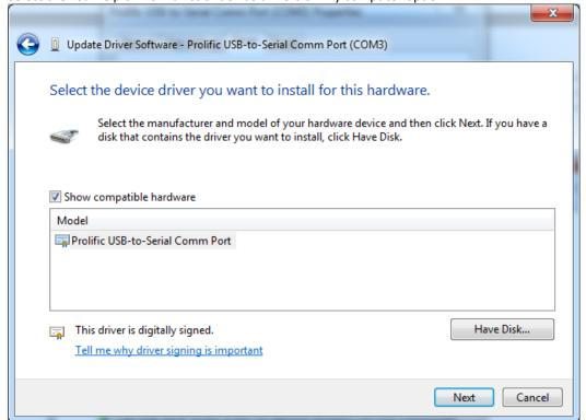
Select the correct driver, and click next. This will install the correct driver. You will need to restart the PC for this driver to be used.
