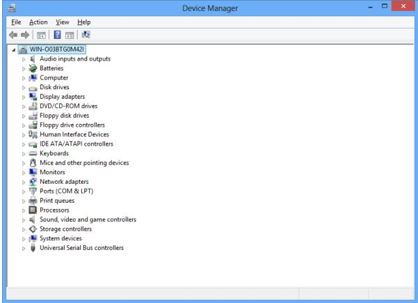
Expand the Ports (COM & LTP) value, which should have a USB Serial Port (COM2) or similar under it.
