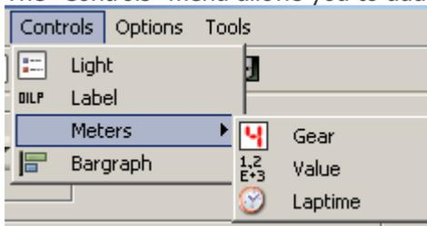
Every control can be dragged with the left button of the mouse everywhere on the screen. To access control properties, click with the right mouse button on the control.
