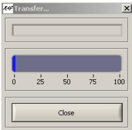
When the upload is finished, the progress bar turns green. You have to restart the dash to display the new configuration.
